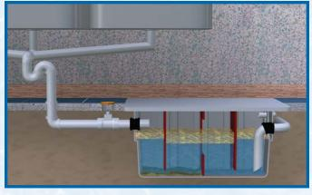
grease to separate, cool to solid form, and collect for removal, prior to it entering a treatment system. Made of 100% corrosion-resistant polyethylene and allows for components to remove easily for cleaning, the FOGHog® retains floatable substances, including: fats, oils, grease, soaps (lanolin) and waxes.
